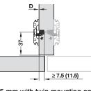
7.5 mm with twin mounting and 11.5 mm with full overlay, half overlay and inset mounting
